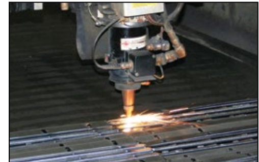
Our 3 available Laser Machines have a 4' x 8' bed and a maximum speed of 6,000 inches per minute. They'll get the job done with speed and accuracy.
