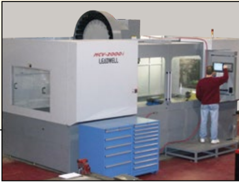
The LEADWELL MCV-2000i is capable of 4-axis milling of large parts up to 40" x 80". Onboard 30-tool changer makes this machine great for both long or short runs.
